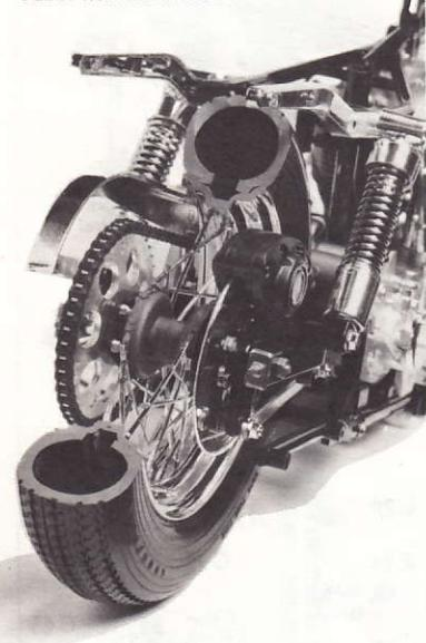
**14** *(Construction of Oil Tank)*
