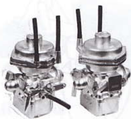
Fig. 17 Construction of Carburettor Each Right Carburettor and Left one has three Vinyl Cords. Check the part number of Carburettor.
