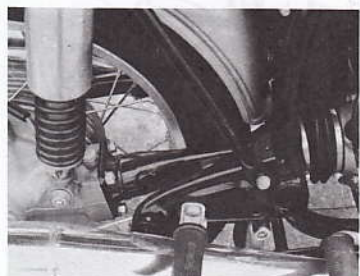
Fig. 12 Construction of Rear Brake Rear Brake is movable through Spring. The position of fixing Brake is the inside of Frame. See the picture below.
