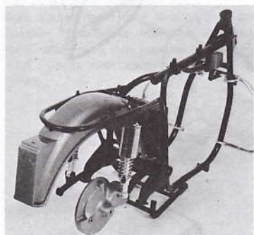
Fig. 12 Construction of Rear Brake Rear Brake is movable through Spring. The position of fixing Brake is the inside of Frame. See the picture below.
