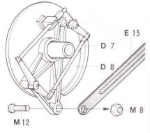
Fig. 18 Installation of Front Wheel
