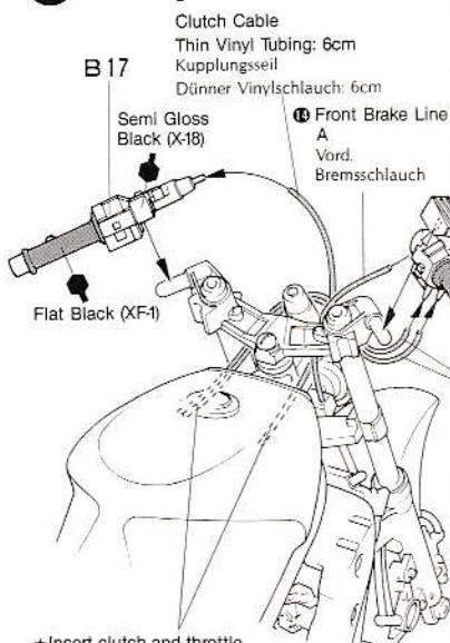
\* Insert clutch and throttle cables into fuel tank.
