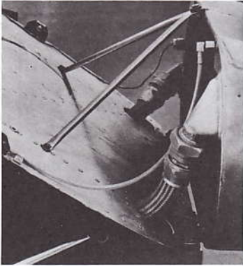
Figure 25. Nose Cowling Assembly. Fasten the nose cowling with the three flat screws provided, as shown in the diagram.
