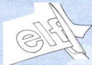
uneven or curved, press the decal down with a hot towel so that the warmed, wet decal will fit the surface well. Cut off the excess transparent portion around a decal before applying. When so done, you can expect a sharp finish with the decal precisely in its specified place.
