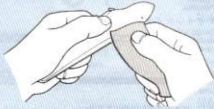
★ Remove dust and oil from all parts prior to painting by washing with detergent. Rinse off thoroughly and allow to air dry.
